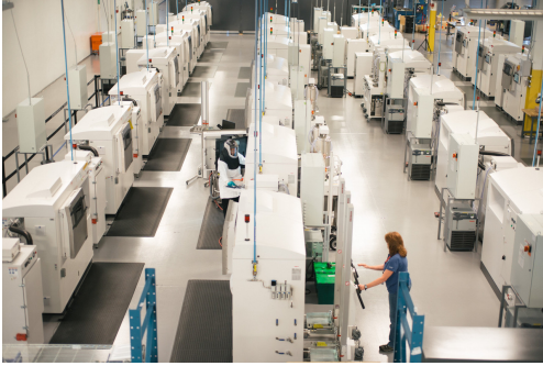
A technician at a General Electric plant in Auburn, Ala., monitors a 3-D printer while it builds a jet-engine nozzle. GE picked Auburn for the printers partly because of access to Auburn University for research projects. PHOTO: BOB MILLER FOR THE WALL STREET JOURNAL
